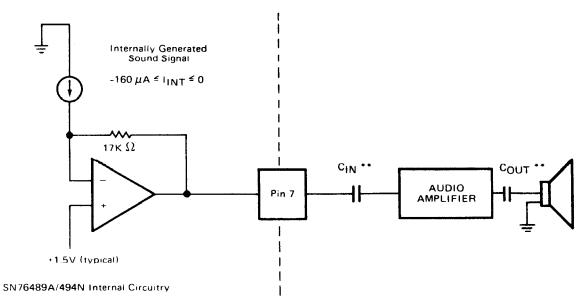
\* These capacitance values are determined by the frequency response desired and the audio amplifier used.
